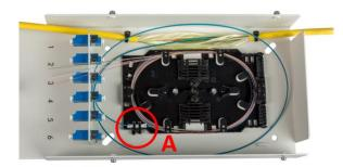
For Tight Buffer pigtails measure the length of the  $900\mu$  buffer needed on the splice tray and fix the fibre in the comb (B) of the splice tray.
