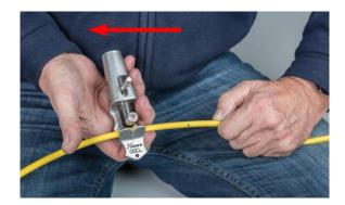
6. Set the tool in the circular cutting mode using D (pull + turn).
