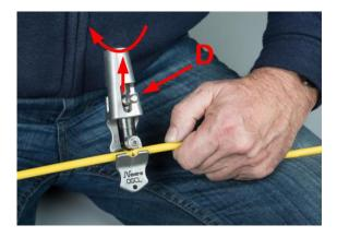
Cut the jacket longitudinally between the 2 marks using the part of the tool dedicated to this operation.
