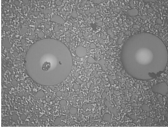
Dust contamination (MPO connector)
