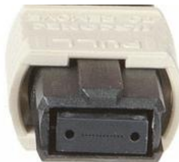
Unpinned MPO connector
