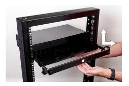
c. When reaching the end of the chassis, lift the drawer further to unhook it. Now both parts can be separated.
