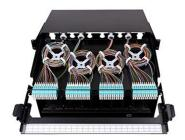
Take the fibre out of the loop rings and mount the connectors on the fibre. When mounting connectors on 250  $\mu$  fibre, you will need to use an optional microtube (N890.045) to reduce risk of damaging the fibre. Refer to the 'Anaerobic OF toolkit: N102.230 – Revision C' NCS Installation Guides for detailed information.
