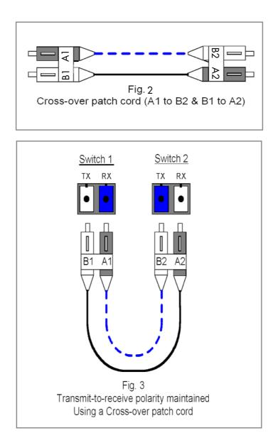
New Nexans LANmark-OF patch cords (DSC, DLC, MT-RJ) produced from Q4 2004 are compliant with the Cross-over concept.
