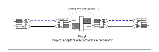
MT-RJ adapters are also designed to provide a crossover.
