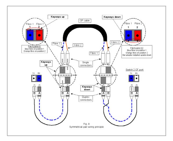
The disadvantage of this principle is that the installer will have to mount the adapters in the opposite way (Upside down) on one side of every OF link.
