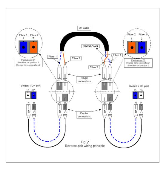
Using this principle is recommended as Data networks are now mainly using duplex transmission channels (Example: Ethernet network). Both ends of a fibre link are not connected to the symmetrical position of the termination patch panels: the fibre n°1 (Blue) is connected on position n°1 of the patch panel on one end and on position n°2 of the patch panel on the other end.
